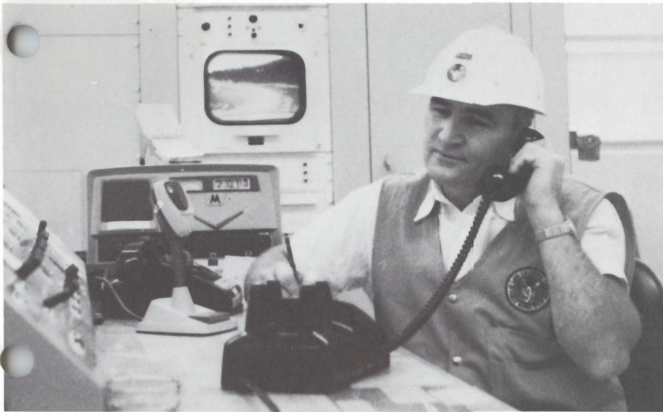
The coming era of the totally automated highway is beginning to show itself in a number of electronically instrumented traffic control systems now being used in and near large cities. Typical is this lane control installation in which monitor at left observes traffic on closed-circuit TV then automatically changes sign at right to give drivers warning well in advance.
